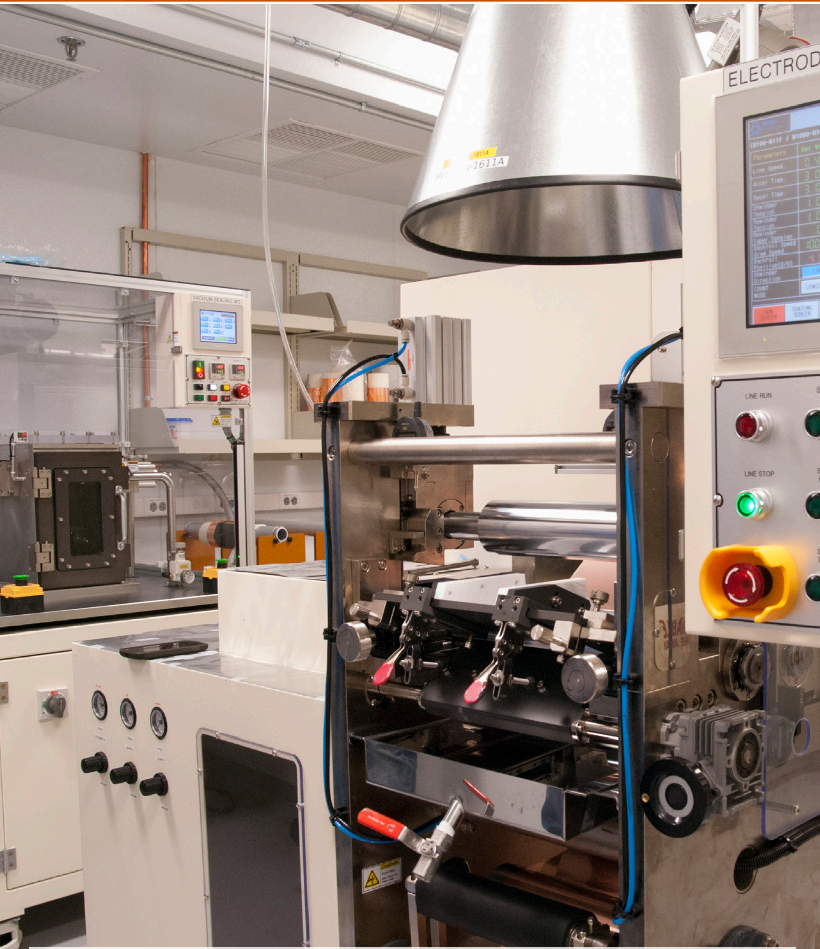
Designed to enable continuous coating/casting of electrode material on either copper or aluminum foil. Capable of double-sided coating for either continuous or segmented electrode films.
