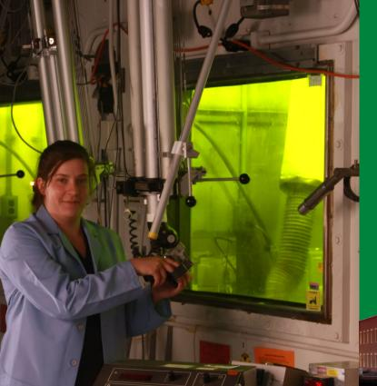
At the Pacific Northwest National Laboratory's Radiochemical Processing Laboratory (RPL), researchers conduct analytical research on nuclear materials using hot cells that shield the researcher from the radiation. The RPL, with its state-of-the-art equipment and instrumentation, is a cornerstone of PNNL capabilities that facilitates cutting-edge science with nuclear materials.
