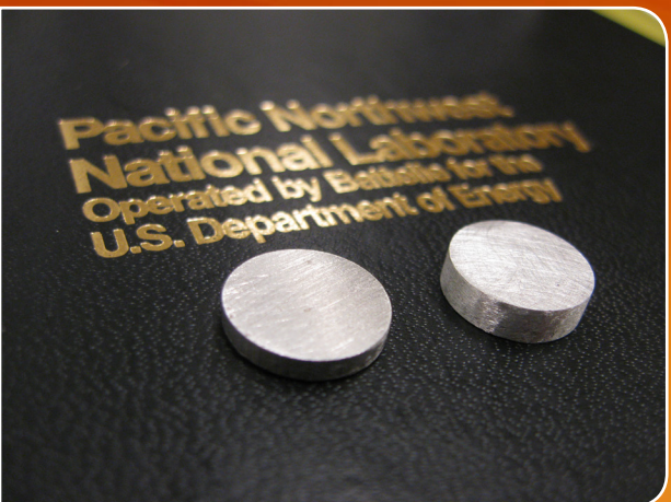
Photo shows magnesium ingots produced via decomposition of dibutylmagnesium through proprietary process
