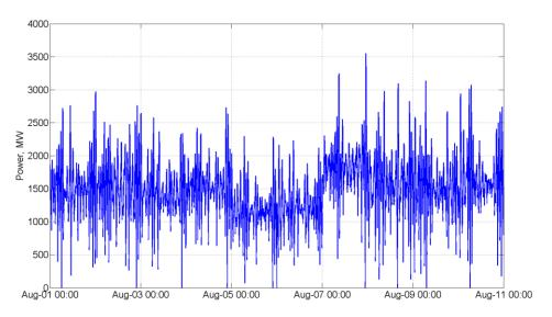
Figure 1. Balancing signal for 14.4 GW of wind generation in NWPP
