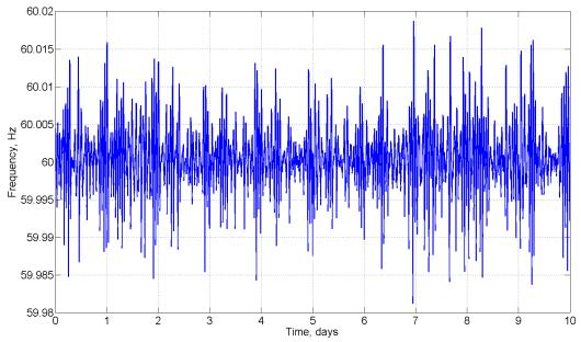
Figure 3. Grid frequency from balancing signal
